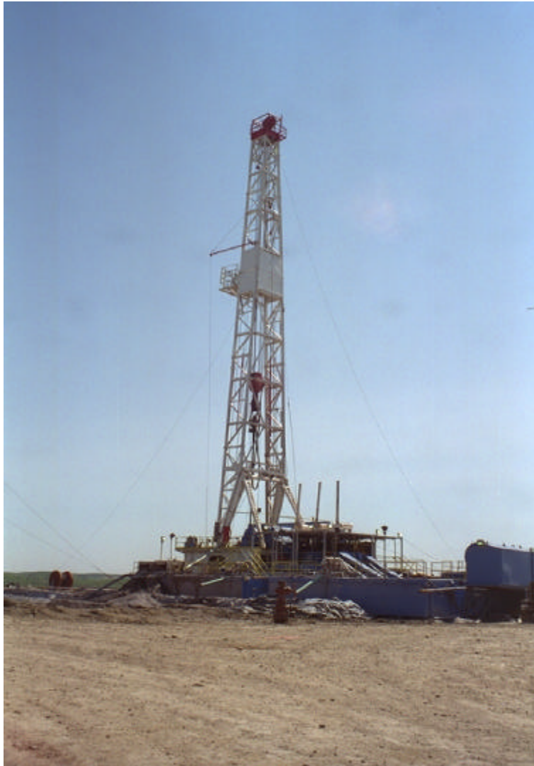
Steuben County, New York, Town of Avoca: Avoca Natural Gas Storage's, Mitchell Well No. 3, drilled by Triad. It was spudded on April 23, 1996, and reached a total depth of 11,415 feet. Drilling was completed on this well on July 31, 1996. This well is part of a program to develop a new underground natural gas storage facility which will have the capacity to store approximately five billion cubic feet of natural gas.
