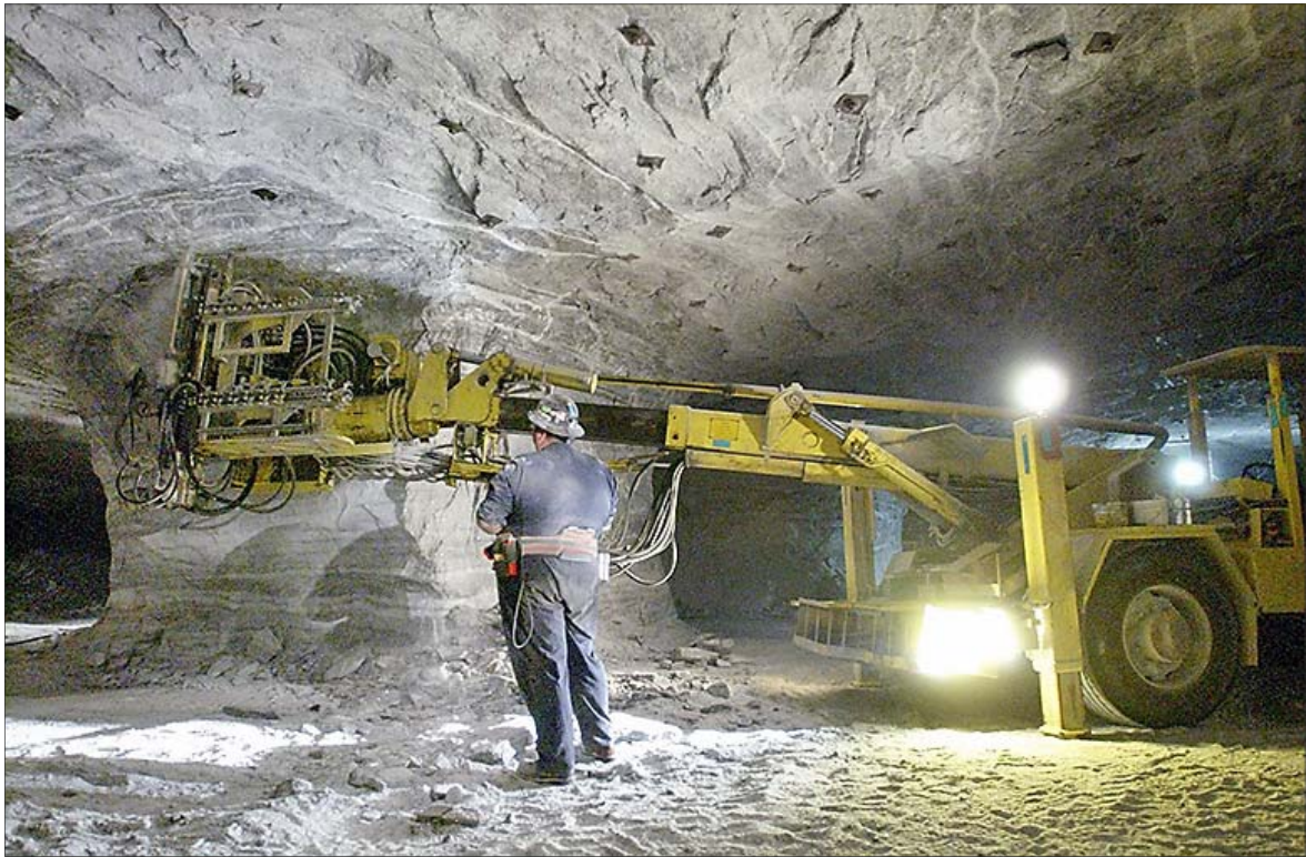
Worker installing roof bolts at Cargill's Lansing Mine. Photograph by Simon A. Wheeler, Elmira Star Gazette 2002, copyright 2004.
