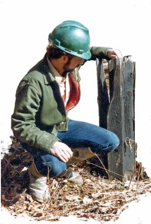
Old wooden casing pulled from a well drilled in the 1800s.
